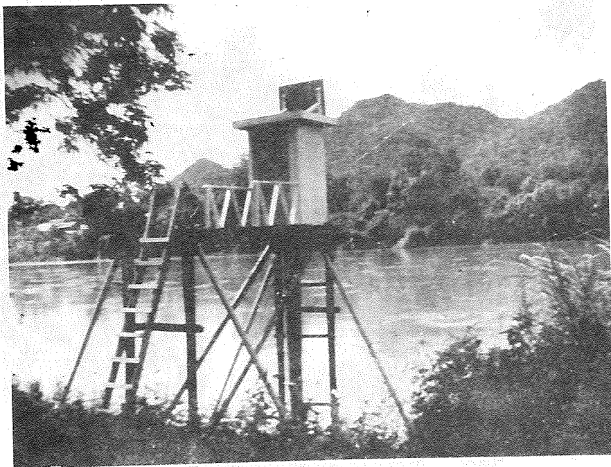
Figure 3. Recording Gaging Station of Mae Klong River at Ban Tham (K.8) Kanchanaburi.
